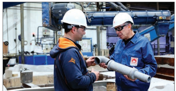
Figure 6: Insulated sprues, runners and ingates create a highly erosion resistant running system.
