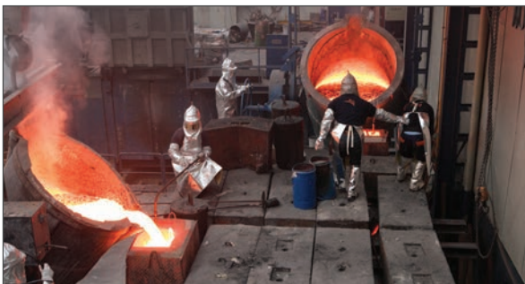
Figure 4: Melt treated with specially designed Foseco fluxes to ensure high cleanliness.
