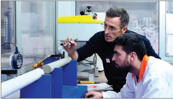
Figure 3: Precision control of reclaimed & new silica sands to prevent mould erosion and dimensional inaccuracy.
