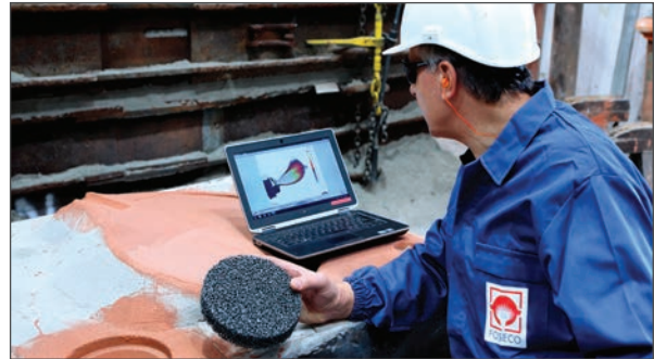
Figure 5: STELEX Pro & SEDEX filters reduce inclusions and eliminate metal turbulence.
