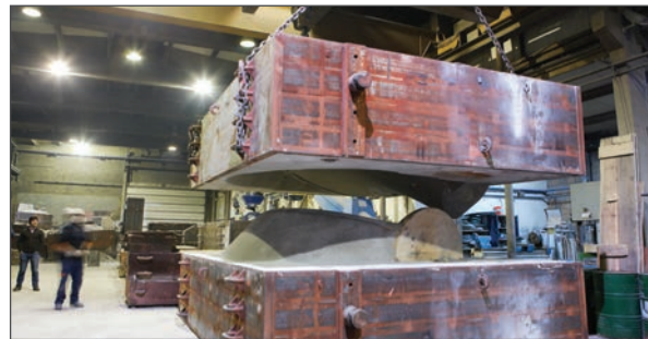
Figure 2: 80% reclaimed sand - 20% new silica sand for the production of perfect moulds.
