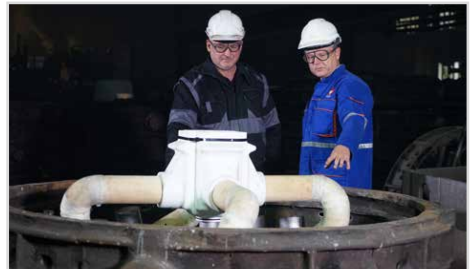
HOLLOTEX Shroud Filter Box during moulding
