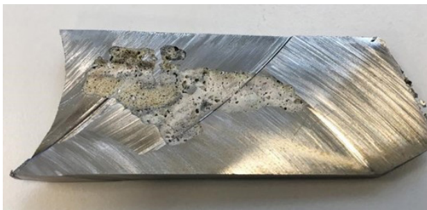
Figure 1. Exogenous non-metallic inclusion in cast steel
