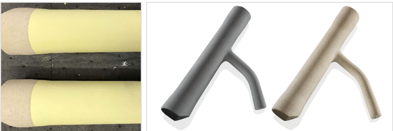
Figure 1: Sand cores manufactured with WASCO* systems and treated with a coating.
