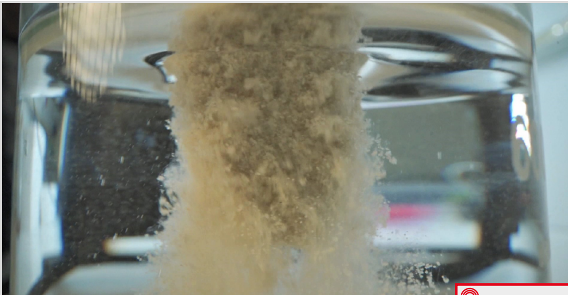
Figure 3: The core solubility shows the clear benefits against conventional core.
