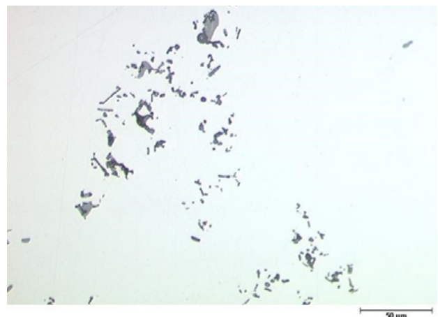
Figure 4. Non-metallic inclusions in cast steel may aggregate into larger clusters.
