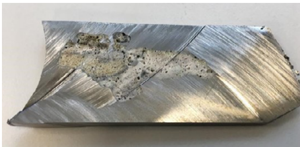
Figure 1. Exogenous non-metallic inclusion in cast steel
