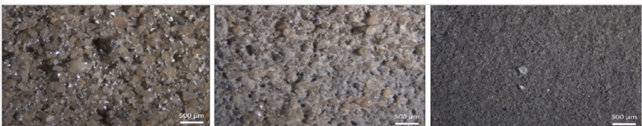
Figure 5: The inner surface of three casting pieces: left – a casting made with an uncoated core; centre – a casting made with the incorrect coating type; right – a casting made with an optimised coating.
