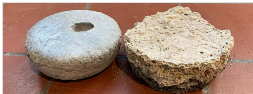
Figure 2: Metal phase and oxide-containing salt phase after dross analysis
