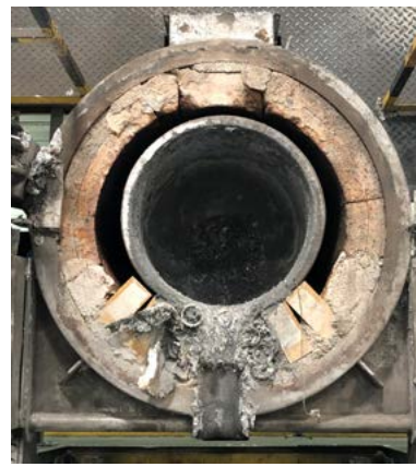
Figure 5: The DURATEK Supermelt after 1284 melt charges.
