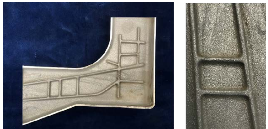
Figure 16: Sand cores with a coating applied by dipping. The coating was furnace dried at 120 °C for 1 h.
