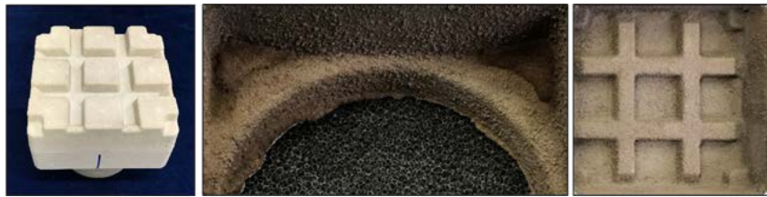
Figure 11: Left: non-coated sand core; middle and right: inner casting surface with significant sand adhesion.
