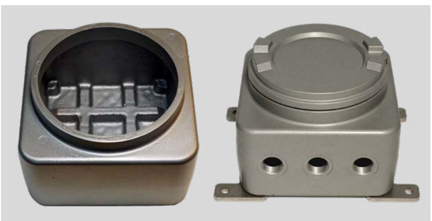
Figure 13: Inner surface of the casting (explosion-proof instrument housing) after removing the coated sand core (courtesy Limatherm S.A. Poland).
