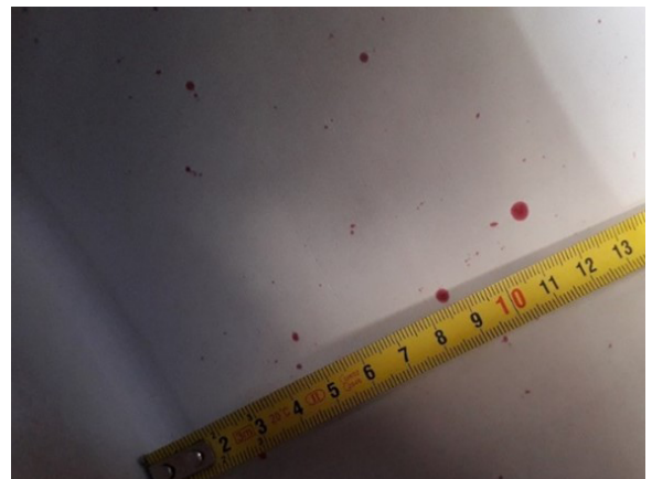
Figure 14b: Defects on the diameter are still present and needs to be further machined
