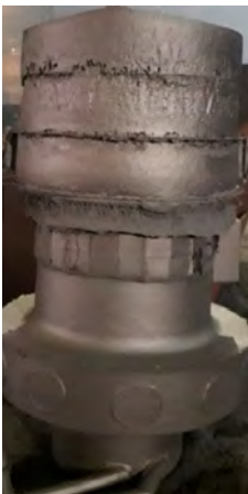
Figure 12a: Shot blasted casting
