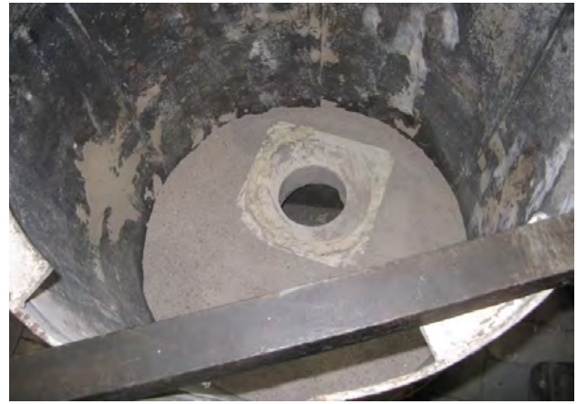
Figure 1. Wellblock L0 installed in the ladle bottom
