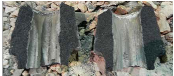
Fig 5. Cross-bore nozzle sectioned after 2 ladle journeys, showing minimum wear of the body material
