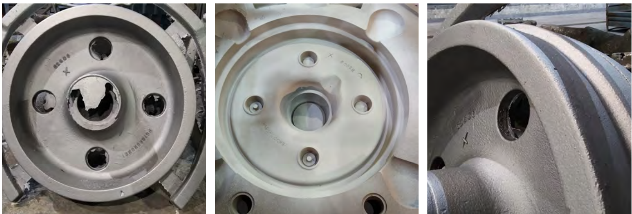
Figure 5. Excellent results in massive castings. Free of burn-on and with good surface quality
