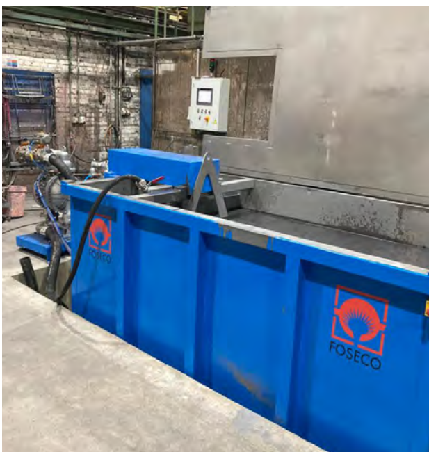
Figure 3: ICU-I - Integrated Density Control and Adjustment in combined Flow Coating and Dip Tank
