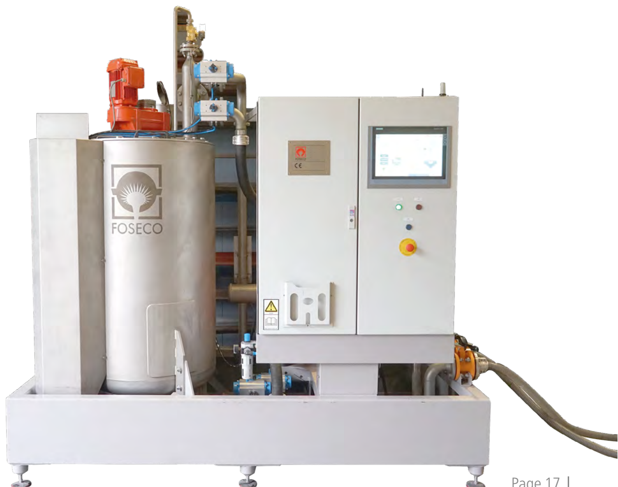
Figure 2: ICU-Pro - Complete coating preparation and application control for water and solvent coatings
