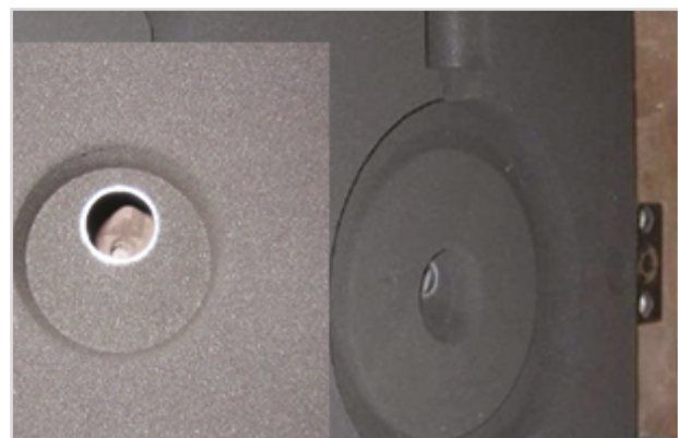
Figure 5. Moulding results on a generic plate casting with collapsible metal breaker core
