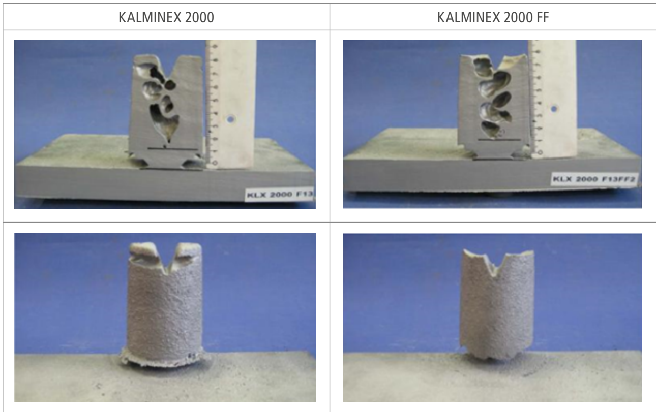
Figure 5a. Ductile iron casting test with KALMINEX 2000 ZP 6/9K/11Q versus KALMINEX 2000 FF FZP 6/9K/11Q on a 250 x 250 x 25 mm plate. Both sleeves showed comparable feed safety margin
