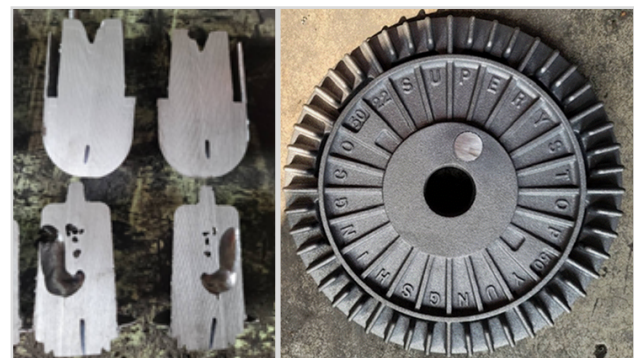
Figure 12 a+b. Photos of section feeders and cast part after feeder knock-off
