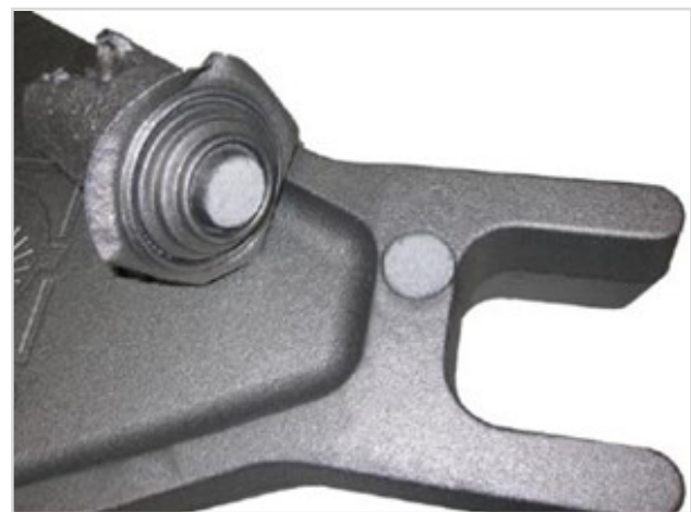
Figure 9. Spot feeder after knock-off, resulting in minimum residual stub
