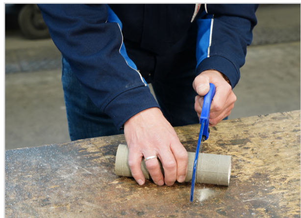
Figure 4. Simple cutting using a hand saw
